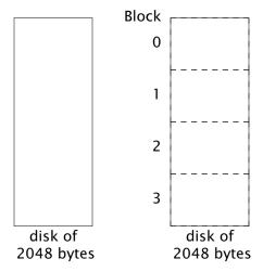
A block is stored to the disk with a tag in the first byte and the Qid.path in the last 8 bytes. The different types of blocks on a disk are: enum
