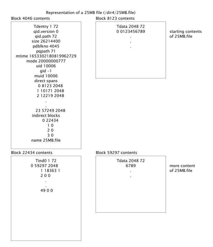
kfs and cwfs do not use Spans. They use blocks but with a size of 8192 bytes to avoid dealing with small data blocks (less system calls, context switches, etc). Hence, they store multiple directory entries (Dentry) per block. They use slot numbers to identify a particular directory entry in a block of directory entries. Instead, we use variable length
