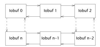
The size of the buffer cache is: number of hash buckets \* collisions per hash bucket \* block size. The approximate size of the buffer cache = Nbuckets \* Ncollisions \* Rawblocksize = 256 \* 10 \* 512 bytes = 1.28GiB. The -h parameter can be used to change the number of hash buckets.
