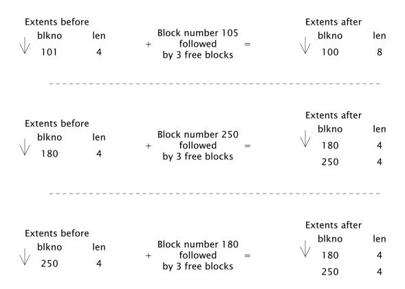
Kfs stores the list of free blocks in a Tfrees block and the Superblock. Instead we use block management routines, similar to pool.h, to allocate and monitor free blocks. On shutdown(), the block management routines (extents.[ch]) store state into the free blocks. This can be read from /adm/frees. On startup, this is read back by the block management routines. On a crash, the fsck can walk the directory structure to identify the free blocks and recreate /adm/frees.
