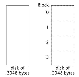
A block is stored to the disk with a tag in the first byte and the Qid.path in the last 8 bytes. The different types of blocks on a disk are: enum
