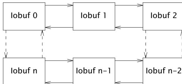
The size of the buffer cache is approximately: number of hash buckets \* collisions per hash bucket \* Maximum Span size. By default, the approximate size of the buffer cache = Nbuckets \* Ncollisions \* Maxspansize = 256 \* 10 \* 1MB = 2.56GB. The -h parameter can be used to change the number of hash buckets.
