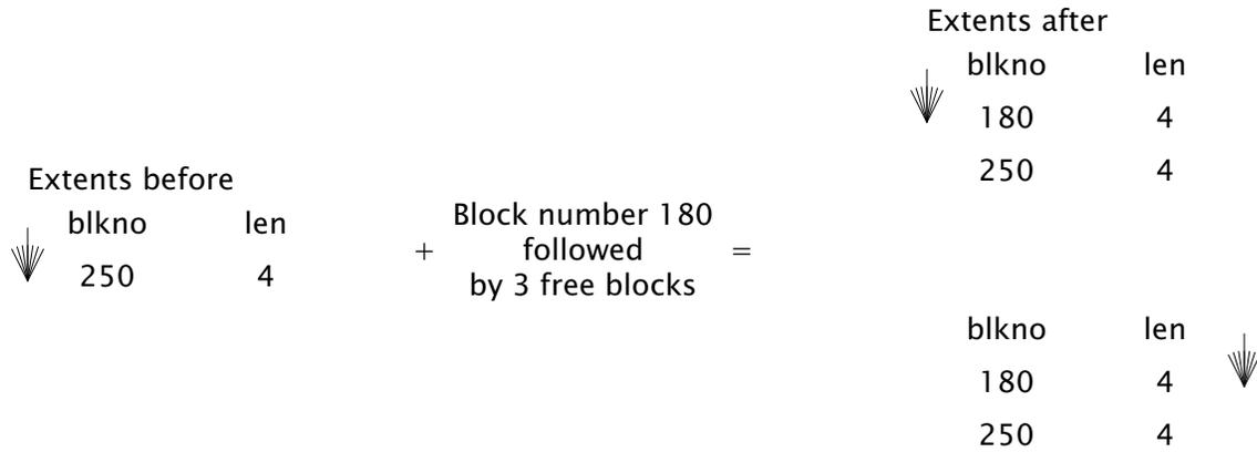
Kfs stores the list of free blocks in a Tfreess block and the Superblock. Instead we use block management routines, similar to pool.h, to allocate and monitor free blocks. On shutdown(), the block management routines (extents.[ch]) store state into the free blocks. This can be read from /adm/frees. On startup, this is read back by the block management routines. On a crash, the fsck can walk the directory structure to identify the free blocks and recreate /adm/frees.
